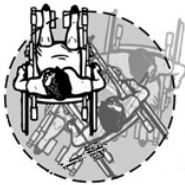
Figure 3: ADA Turn area, 48" minimum
